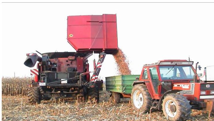
Figure 5 : Tschiggerl Agrar corn cobs harvester
